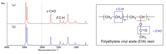
(a) Before photoresistance testing (b) After photoresistance testing Fig.1 Results of FT-IR measurements of EVA resin (VA content 18%) before and after photoresistance testing.
