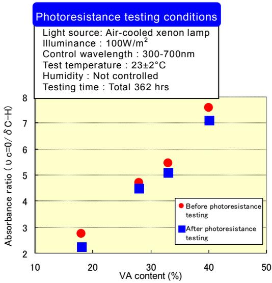
Fig.2 VA content – absorbance ratio before and after photoresistance testing.
