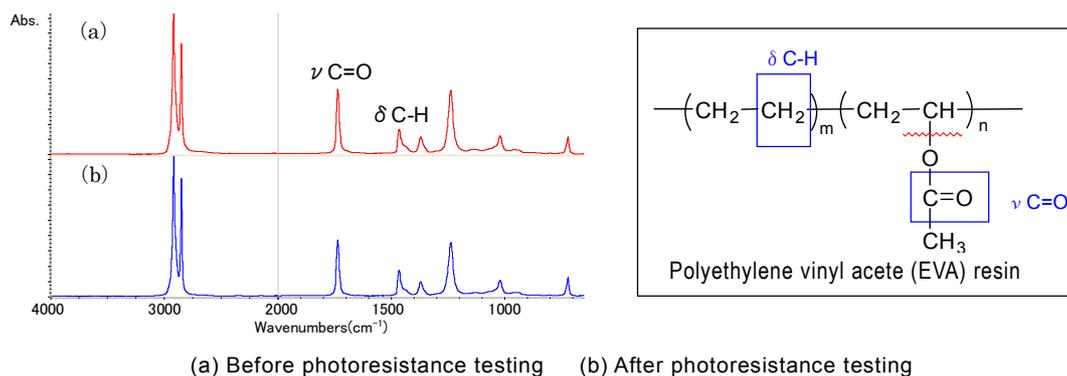
Fig.1 Results of FT-IR measurements of EVA resin (VA content 18%) before and after photoresistance testing.
