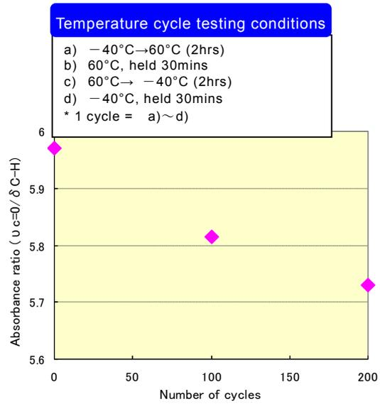
Fig.3 Absorbance ratios before and after temperature cycle testing.
