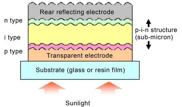
Fig.1 Basic structure of amorphous silicon solar cell.
