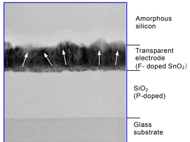
Fig.4 Expanded TEM micrograph of transparent electrode ( $\text{SnO}_2$ ).
