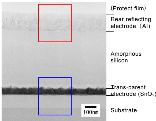
Fig.2 TEM micrograph of cross section of solar cell.
