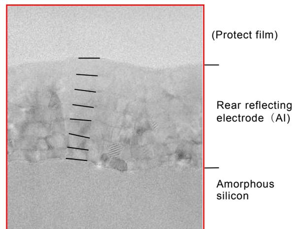
Fig.3 Expanded TEM micrograph of rear reflecting electrode (Al).
