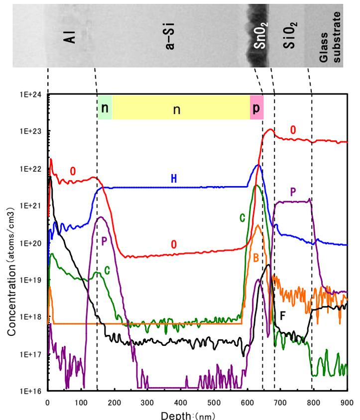
Fig.5 Results of SIMS analysis of amorphous silicon solar cell.
